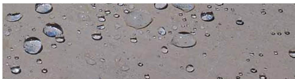
Penetrating Sealers penetrate deep into the concrete to effectively repel water and protect the surface. Most penetrating sealers provide a matt finish.
