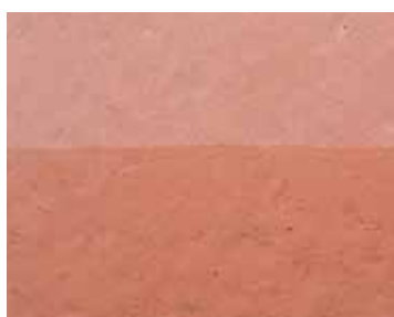
Sealed and unsealed. Sealing concrete with one of the gloss CCS acrylic, epoxy or urethane sealers will give concrete that wet look.
